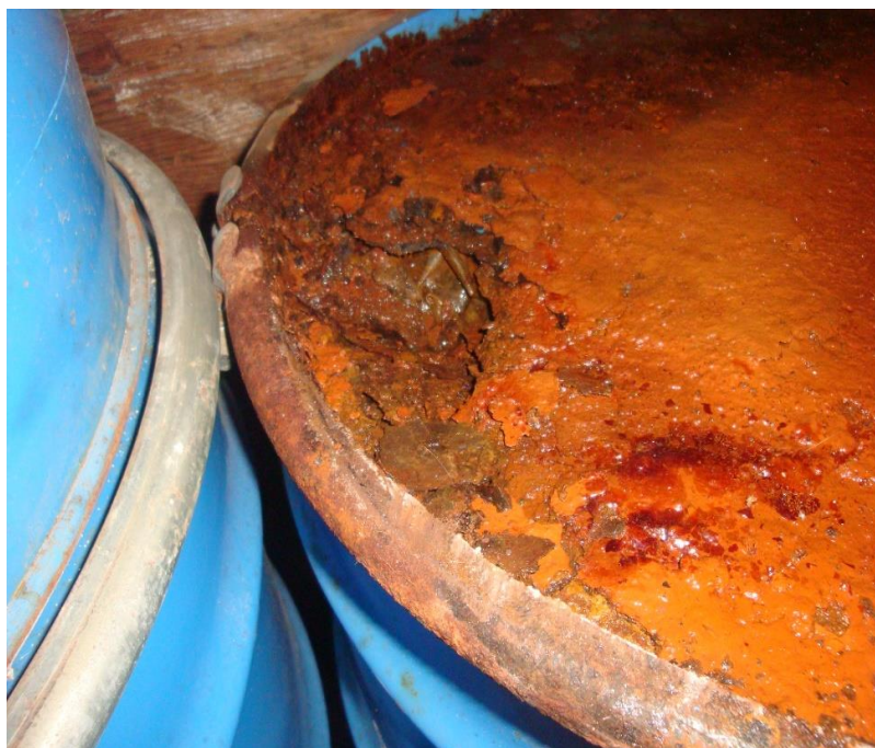
Figure 5. Example of degraded condition of a drum at MoH Belmopan.
