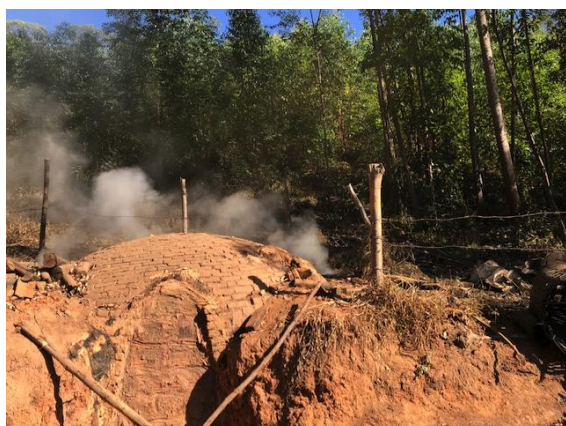
Old fashion kiln - Hillside Kiln ("forno de encosta")
