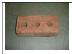
Perforated brick: In India, most of the perforated bricks have 3 holes and have a 5-15% perforation ratio. The size of these bricks is similar to that of normal bricks. The reduction in clay and fuel is small.
