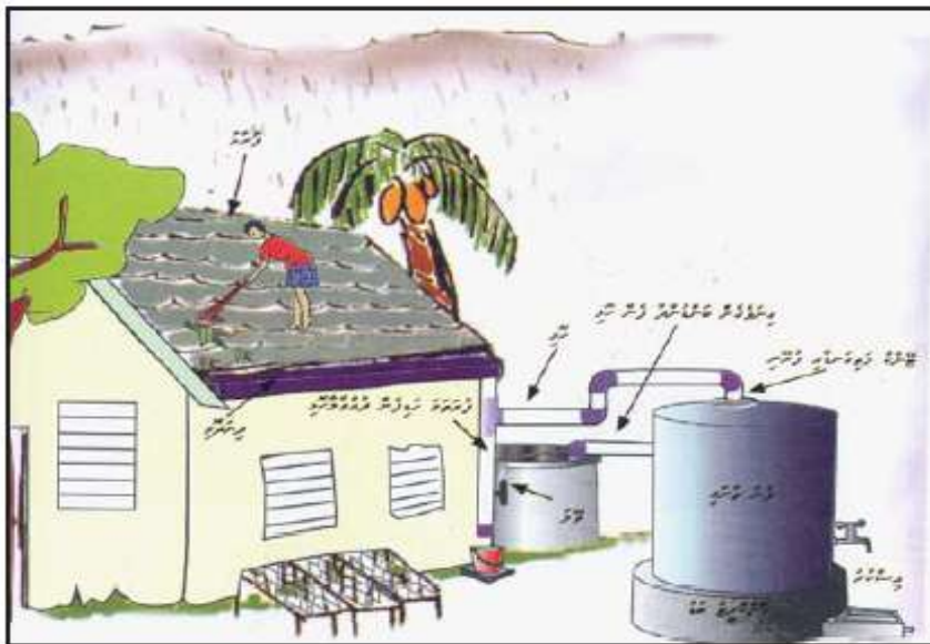
Fig.3: Basic elements of a domestic rainwater harvesting scheme in the Maldivian context (WHO, 2007)
