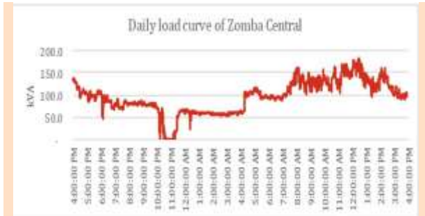
Figure 12 Daily Load curve- Zomba Central
