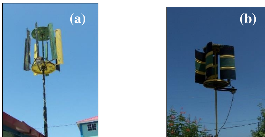
Figure 9 Savonius type vertical axis wind turbine at CMI with (a) PVC pipes as blades and (b) quarter drums as blades.
